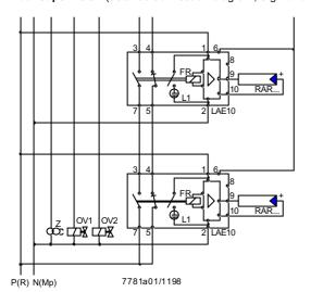
With this type of supervision, **one** flame is supervised by **two** independently operating flame safeguards, aimed at reducing the possibility of loss of flame during operation in case of a simultaneous failure of **both** flame safeguards to an "improbable coincidence".
