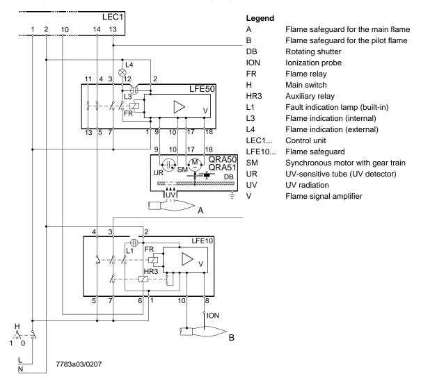
Supervision of the pilot burner (B) with an ionization probe «ION» and a flame safeguard LFE10... until the end of the second safety time is reached.
