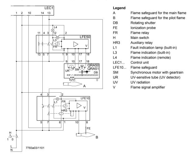
Supervision of the pilot burner (B) with an ionization probe «FE» and a flame safeguard LFE10... until the end of the second safety time is reached.
